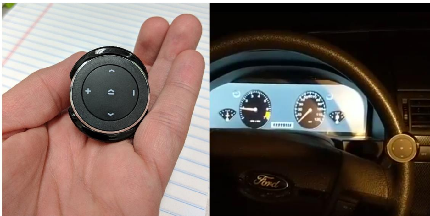
Figure 3. Bluetooth™ push button used to collect subject responses
